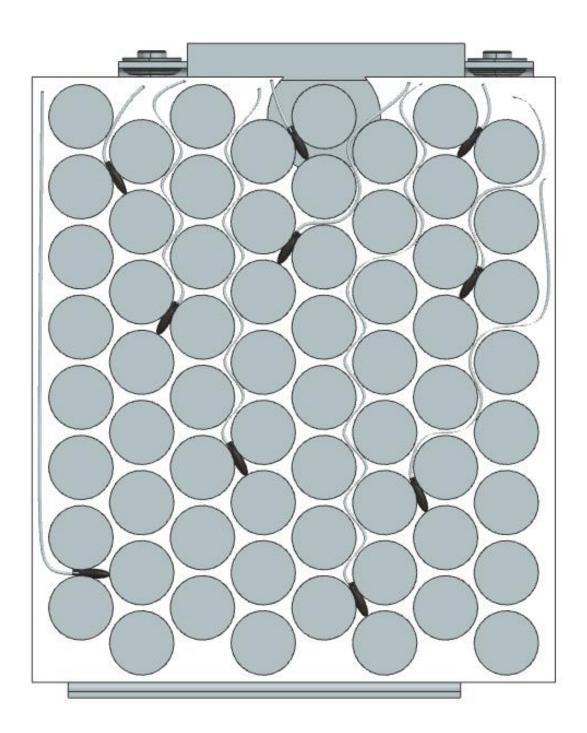
Figure 1: Cell Temperature Sensor Distribution
