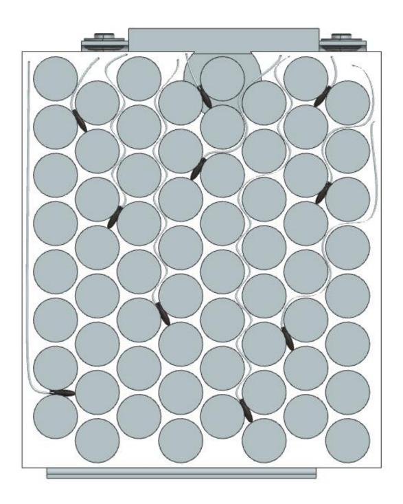
Figure 1: Temperature Sensor Distribution
