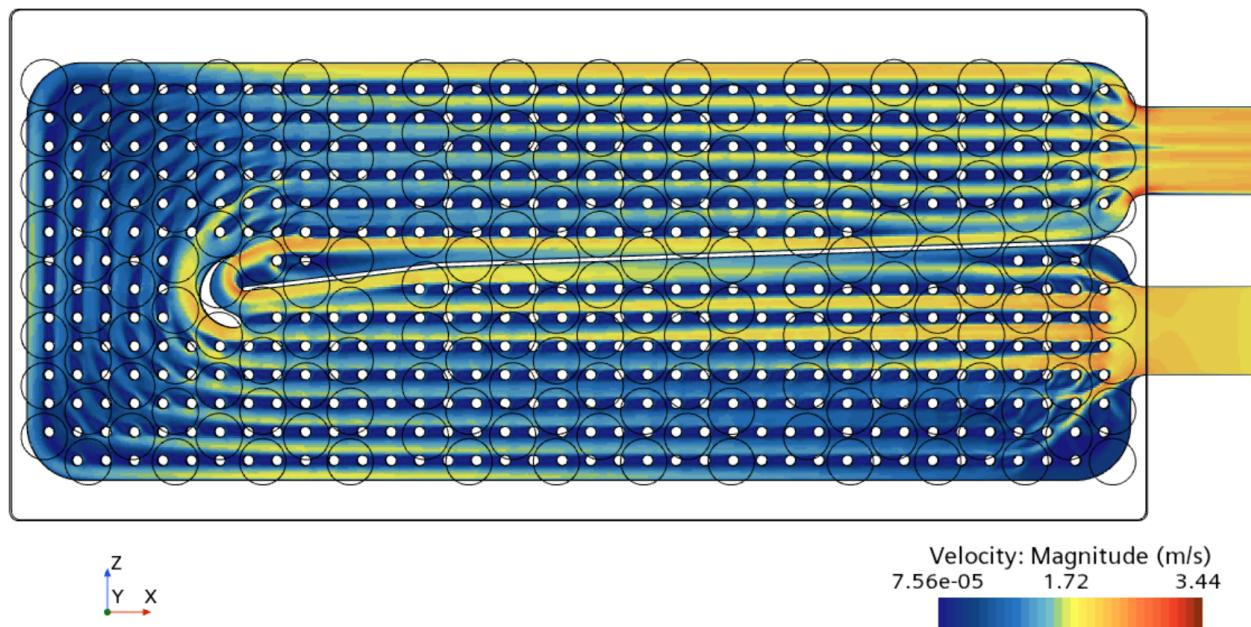
Figure 1: Water Flow Simulation of the Cooling Plate
