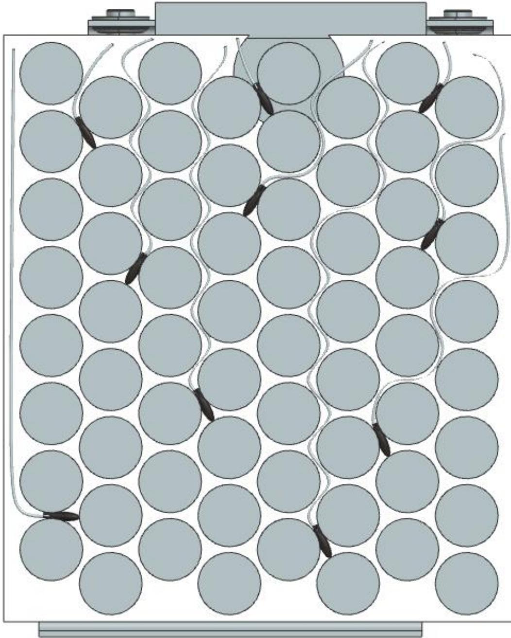
Figure 1: Temperature Sensor Distribution
