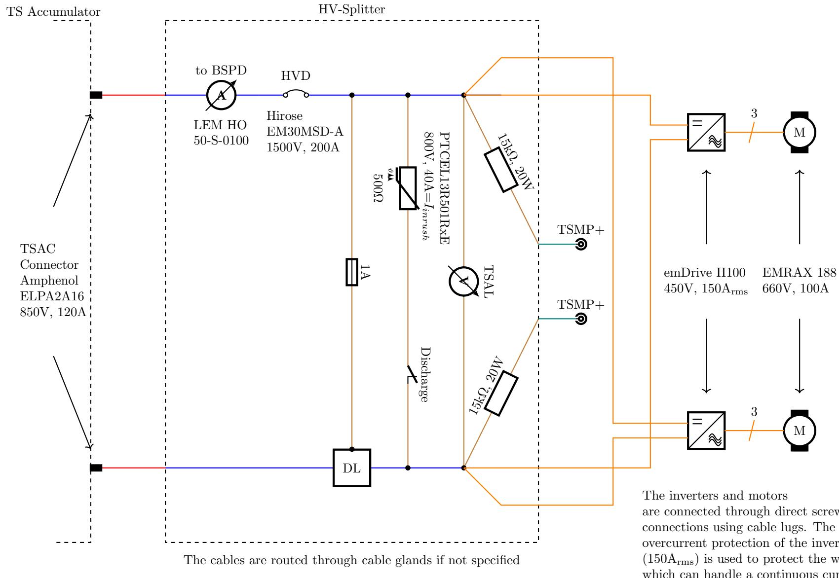
The inverters and motors are connected through direct screwed connections using cable lugs. The built-in overcurrent protection of the inverters ( $150\text{A}_{\text{rms}}$ ) is used to protect the wires, which can handle a continuous current of 170A.
