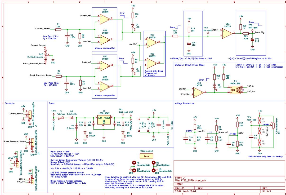
Figure 1: Schematic of BSPD
