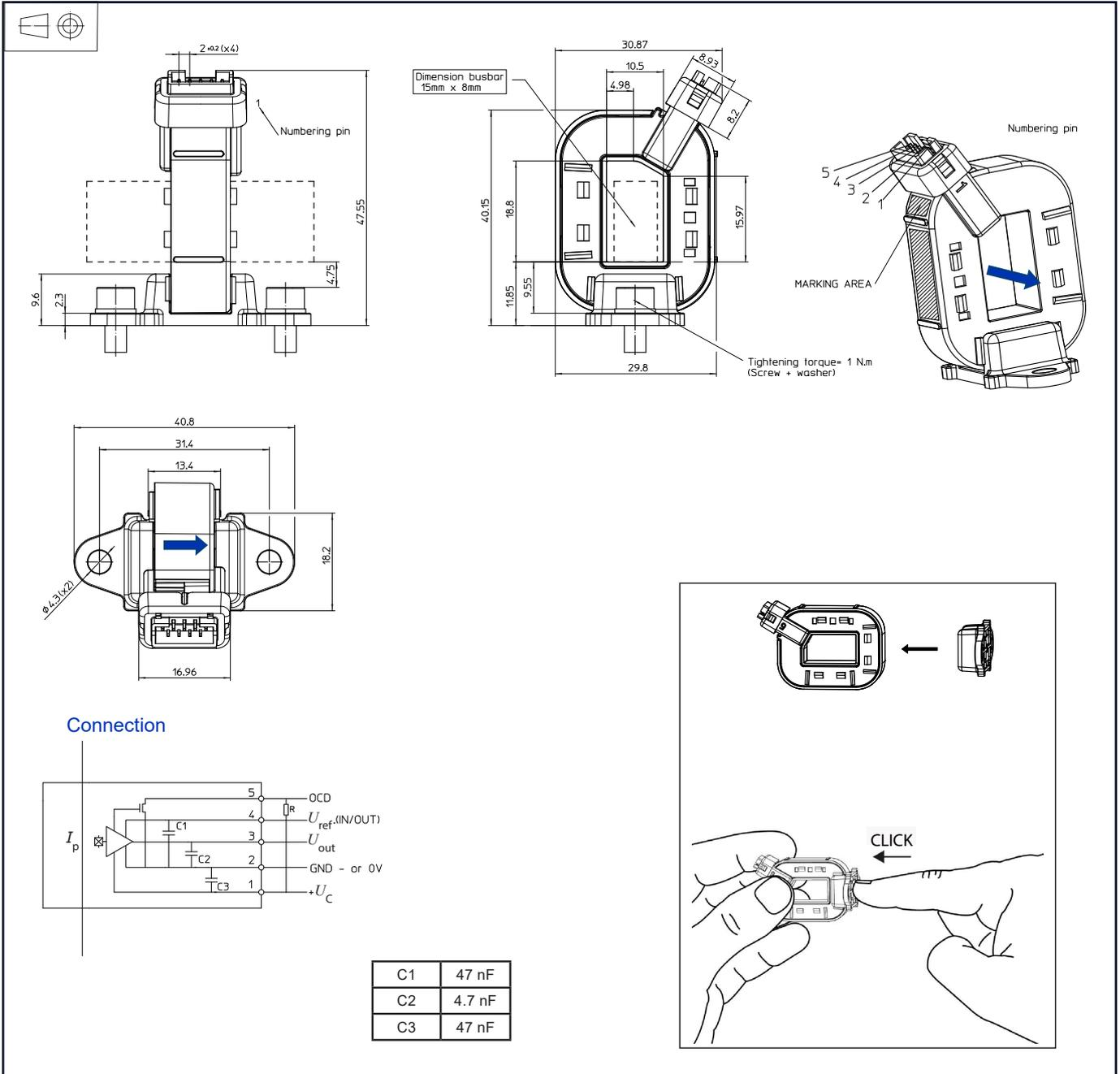
Technical drawing showing dimensions and mounting details for the HO-S series transducer. Dimensions are in mm.
