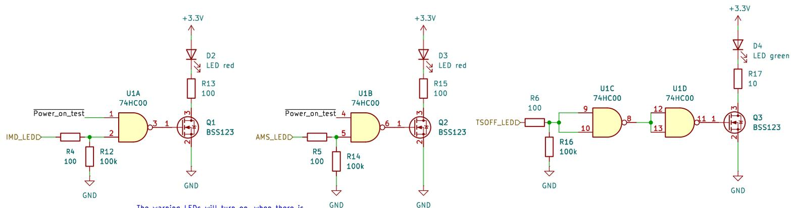
The warning LEDs will turn on, when there is no input Signal or when the cabel for the Signal is shorted to ground or disconnected. Initially the LEDs for the AMS and the IMD will turn on, to show the functionality of these.
