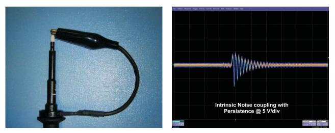
Figure 6. Ringing Voltage Pick-up by 3-Inch Ground Wire
