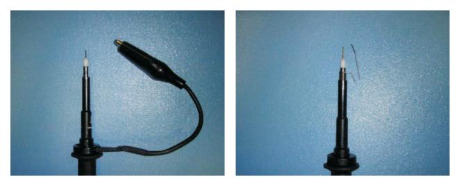
Figure 8. Oscilloscope Probe Comparison: Typical 3-Inch Wire (Left) Versus Small Length Wire (Right)
