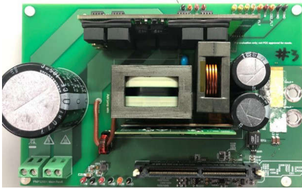
Figure 40. 54-V, 3.6-kW PSFB reference design.
