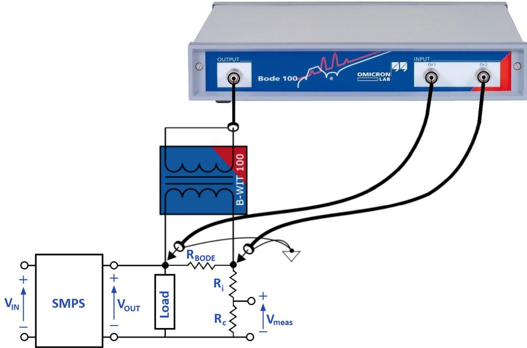
Figure 6-9: Bode analyzer loop stability test setup
