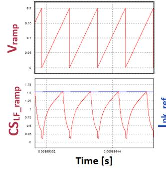
Figure 4-11: Slope compensation
