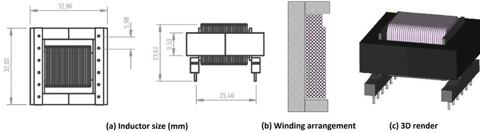
Figure 5-10: Output filter inductor implementation
