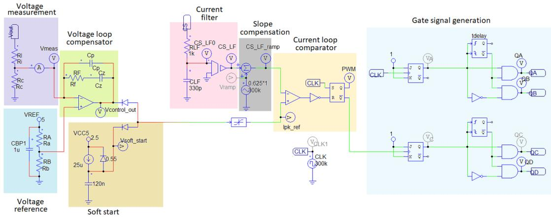
Figure 4-7: Simulation-3: Closed loop control circuit
