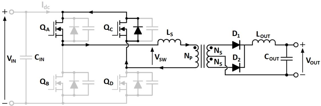
Figure 2-11: Clamped freewheeling interval:  $t_1 < t < t_2$
