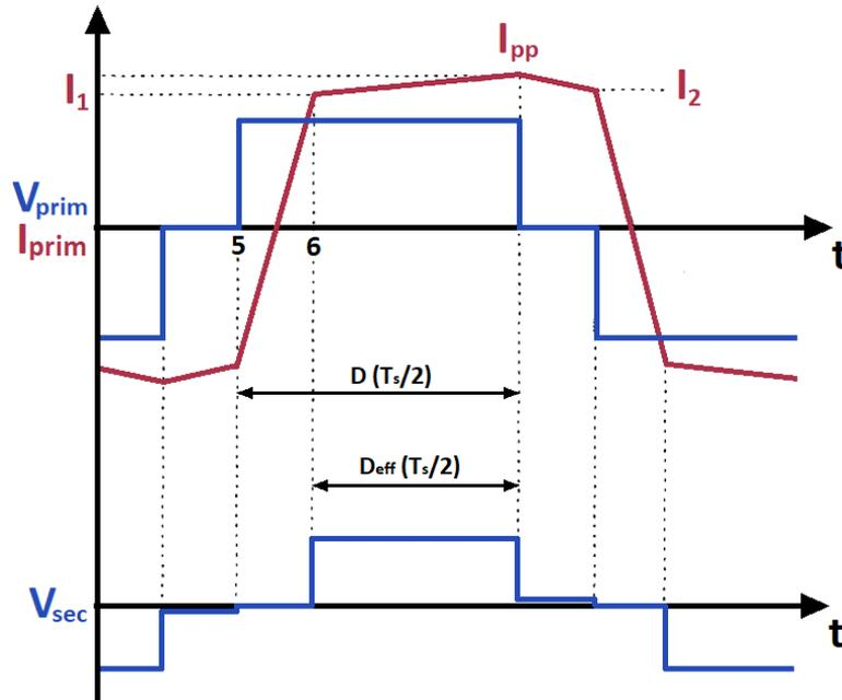
Figure 2-15: "Lost duty": Current and voltage waveforms
