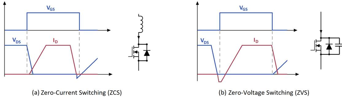
Figure 1-4: Soft switching circuit transients
