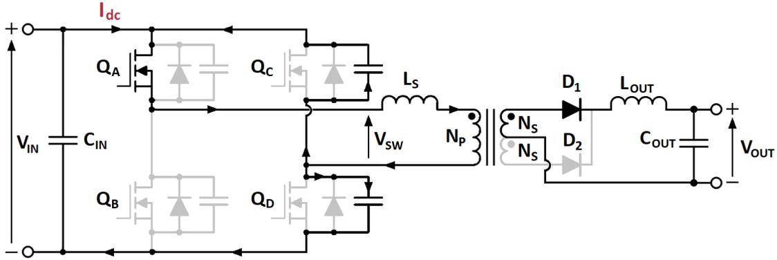
Figure 2-10: Right leg transition:  $t_0 < t < t_1$
