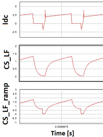
Figure 2-18: Current measurement and ramp compensation
