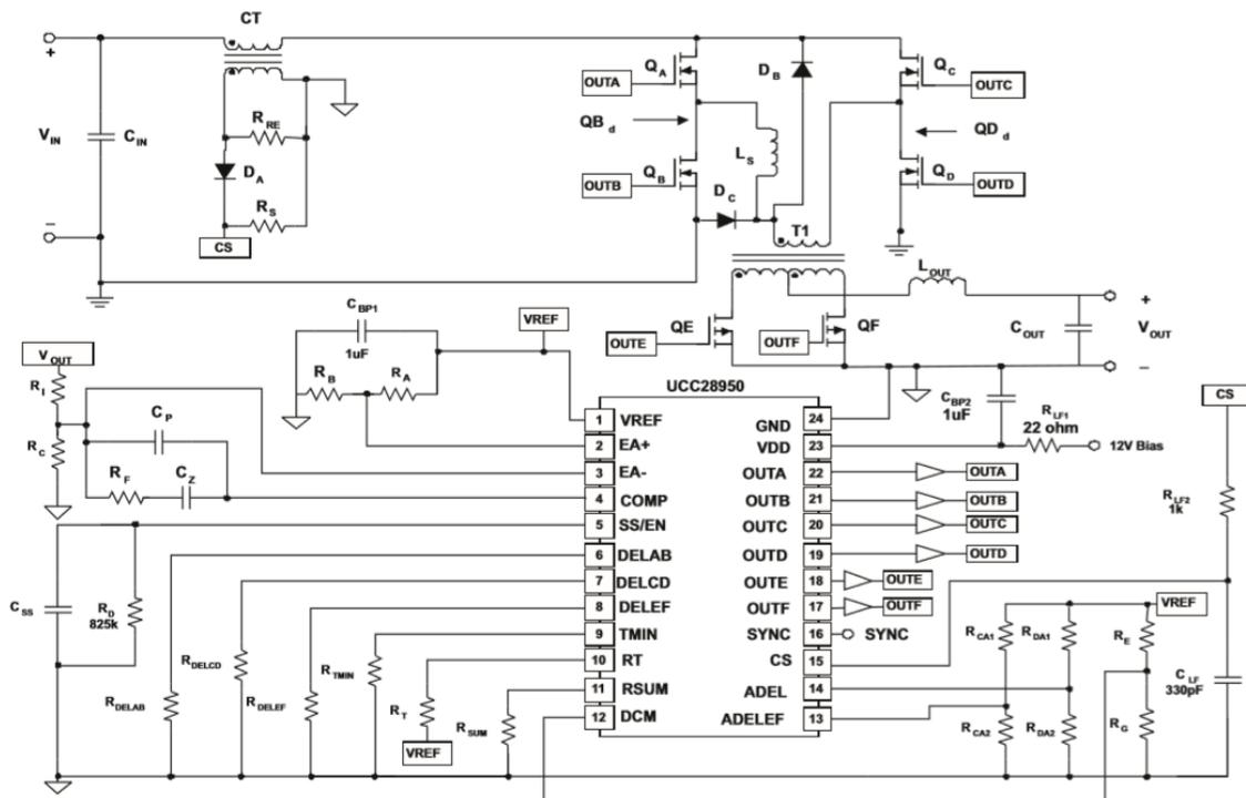
Figure 3-4: UCC28950 Phase-Shifted, Full-Bridge Functional Schematic [9]
