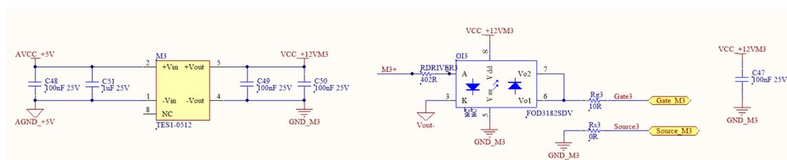
Figure 5-3: Schematic of the driver circuit in Altium Designer
