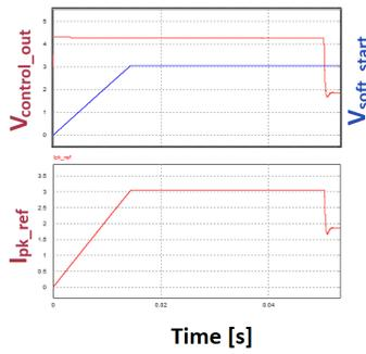
Figure 4-9: Soft starting waveforms
