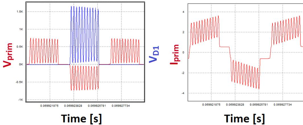
Figure 4-3: Current and voltage waveforms with diode parasitic capacitance
