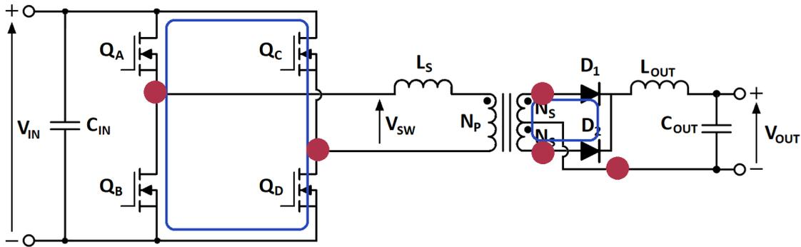
Figure 5-4: High  $di/dt$  loops and high  $dv/dt$  node
