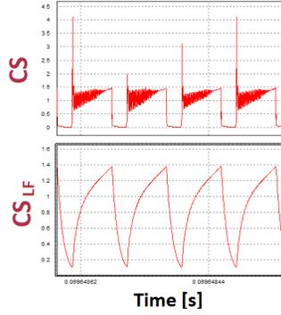
Figure 4-10: Current measurement filtering
