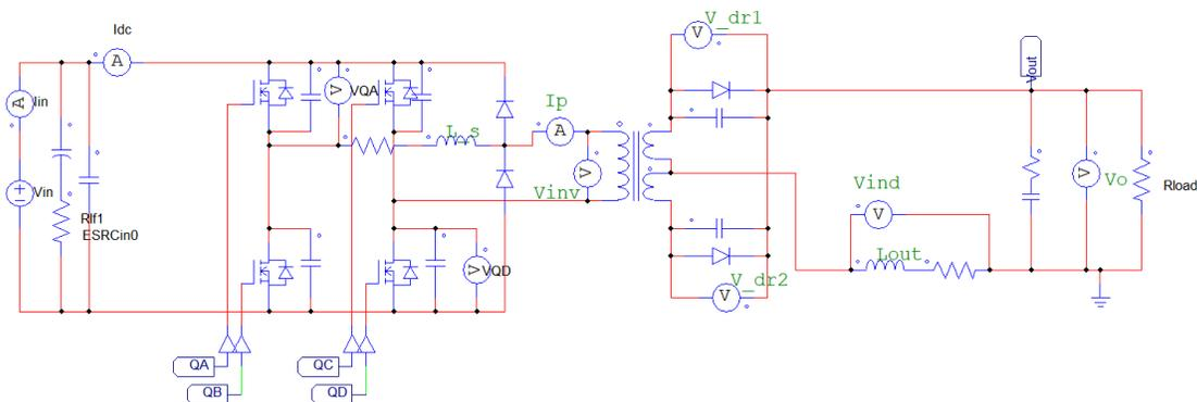
Figure 4-4: Simulation-2: Power circuit with added snubber diodes
