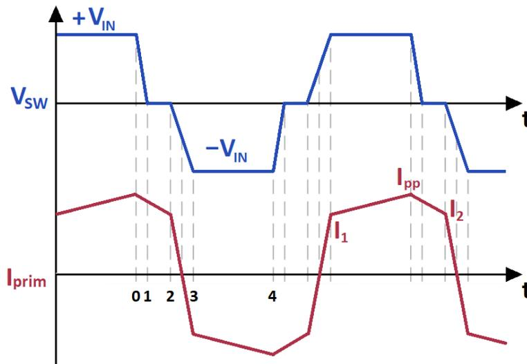
Figure 2-14: Voltage and current wavforms  $t_0 < t < t_4$
