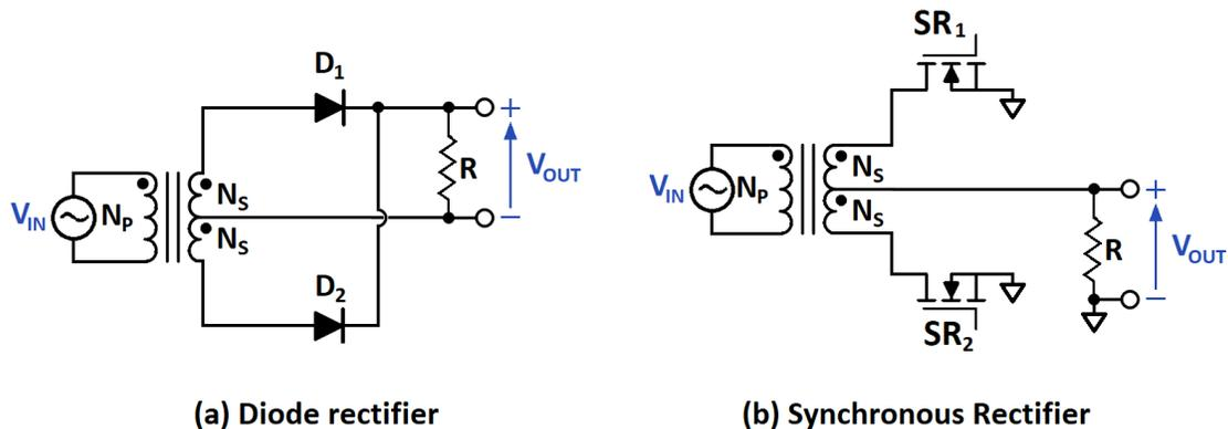
Figure 2-8: Diode rectification vs. Synchronous rectification
