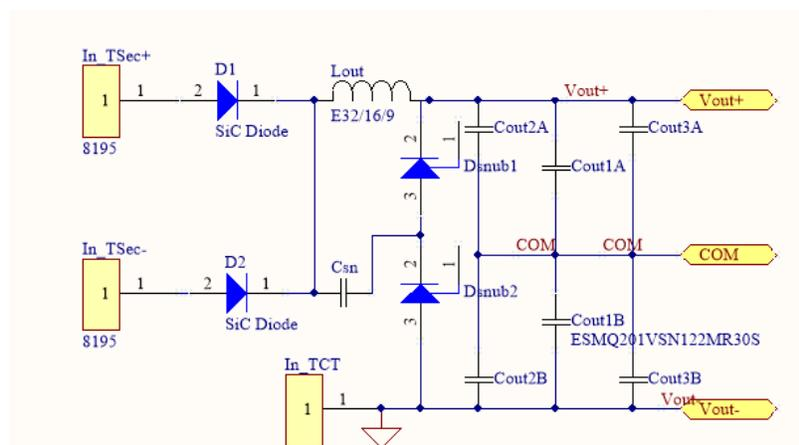
Figure 6-3: Secondary side snubber circuit
