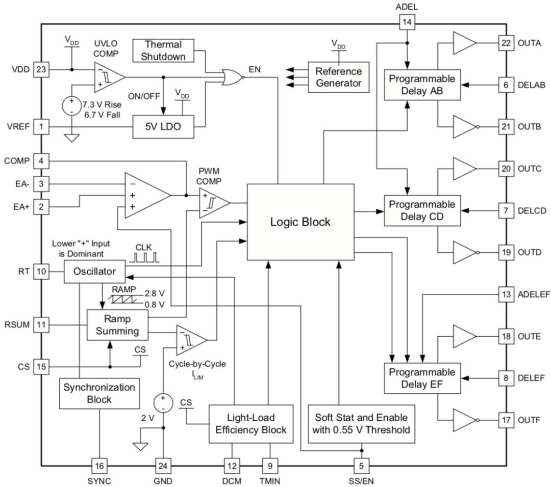
Figure 3-5: Functional Block Diagram of UCC28950 [12]
