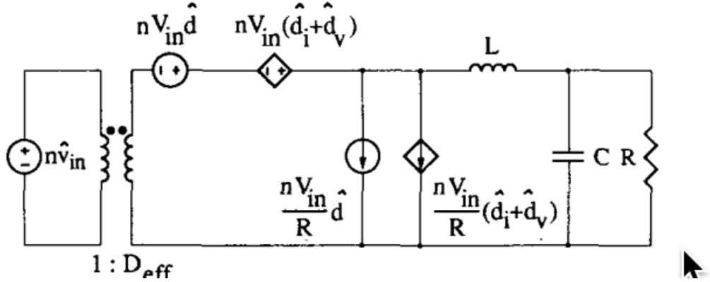
Figure 2-16: Small-signal circuit model of PSFB converter [14]
