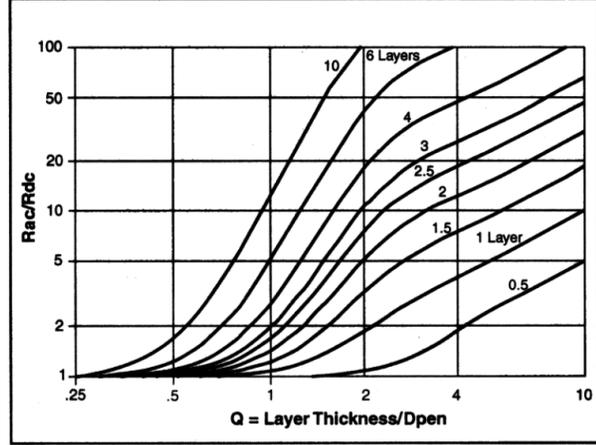
Figure 3-3: Dowell's curves for AC and DC winding losses [11]
