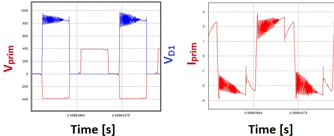
Figure 4-5: Current and voltage waveforms with added snubber
