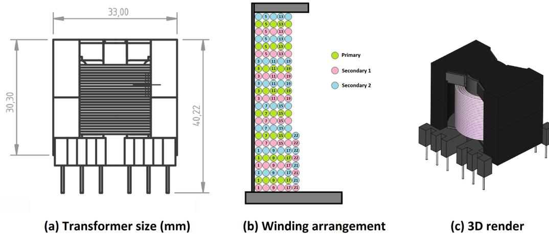
Figure 5-7: Transformer: (a) Coil Former (b) Winding arrangement (c) 3D render
