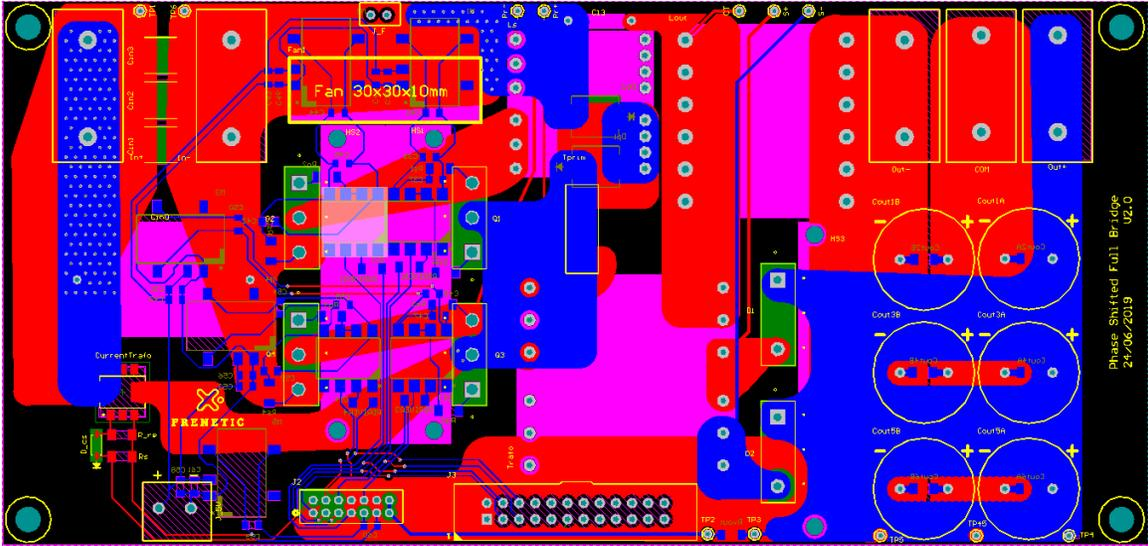
Figure 5-5: Power stage PCB layout on Altium Designer
