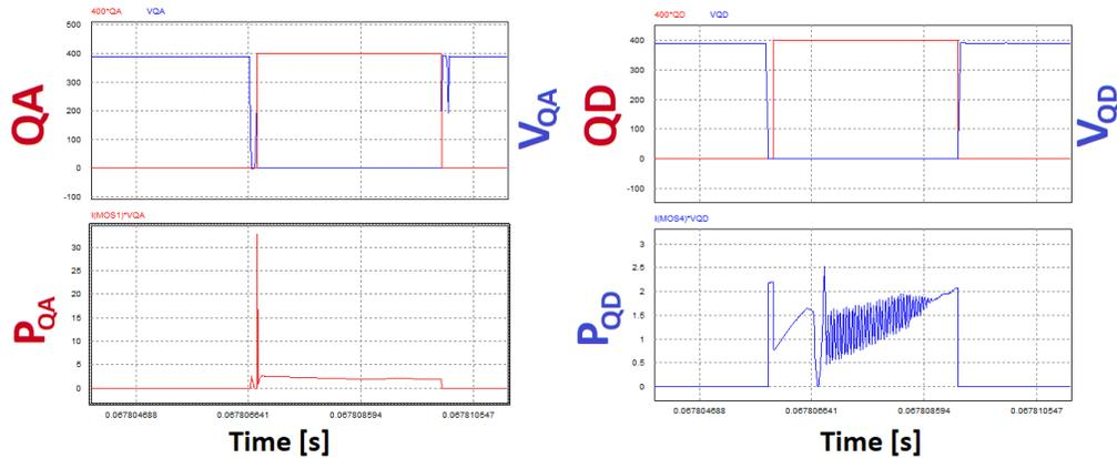
Figure 4-13: Switching transients and instantaneous power losses of leading and lagging leg MOSFETs
