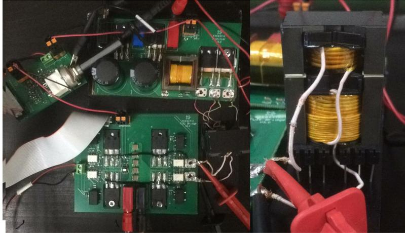
Figure 6-4: PCB-3 using merged transformer and shim inductor
