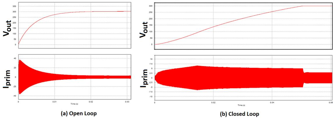
Figure 4-8: Comparison of primary current and voltage transients
