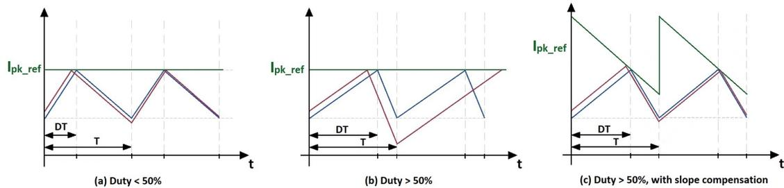
Figure 2-20: Slope compensation on switching inductor current
