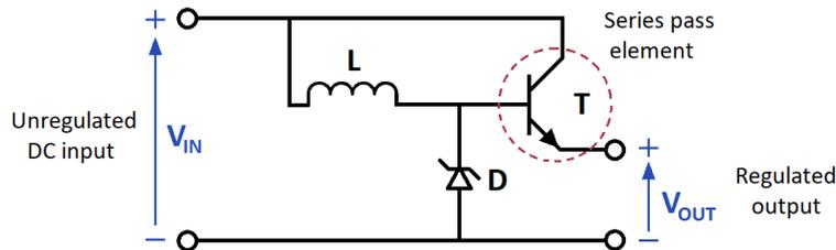
Figure 1-1: Schematic of a linear voltage regulator
