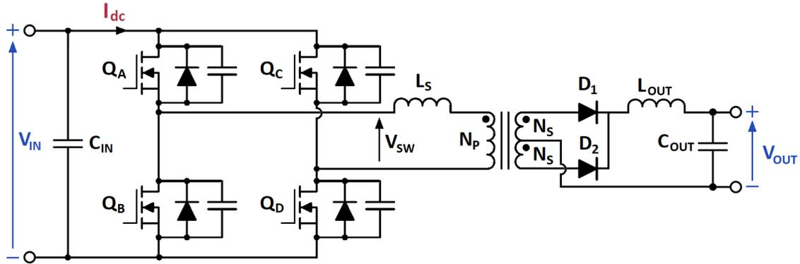
Figure 2-5: Phase-Shifted Full-bridge converter
