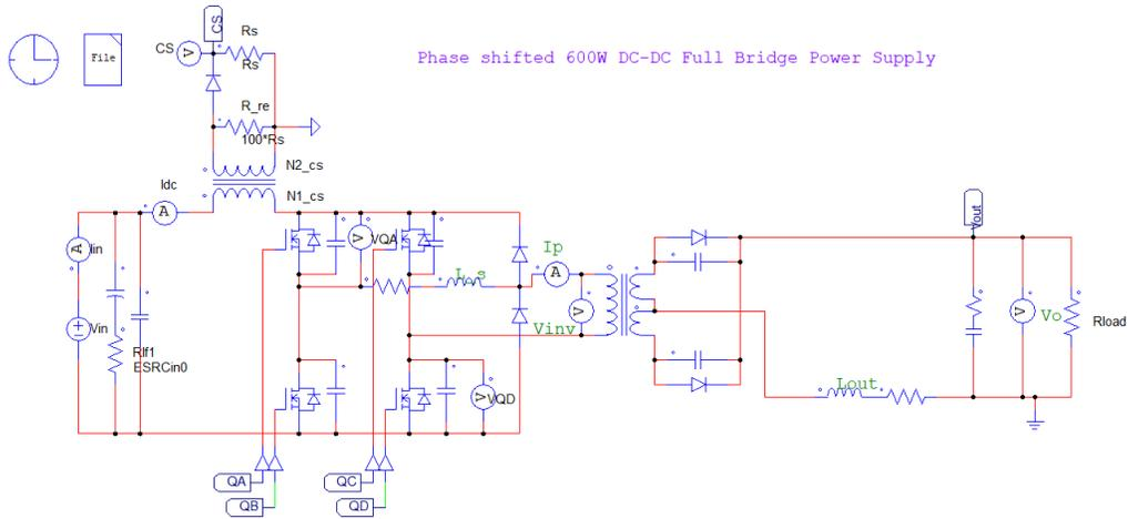
Figure 4-6: Simulation-3: Power stage
