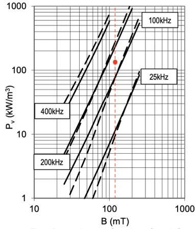
Figure 3-2: Power loss as function of peak flux density
