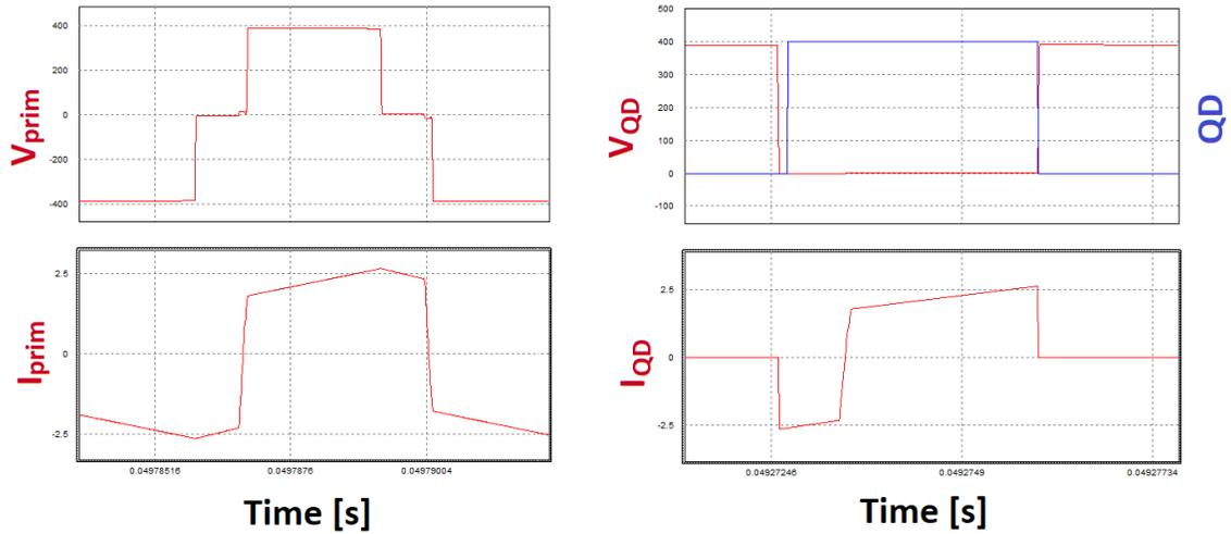
Figure 4-2: Simulation-1: Primary current and voltage, and switching of QD
