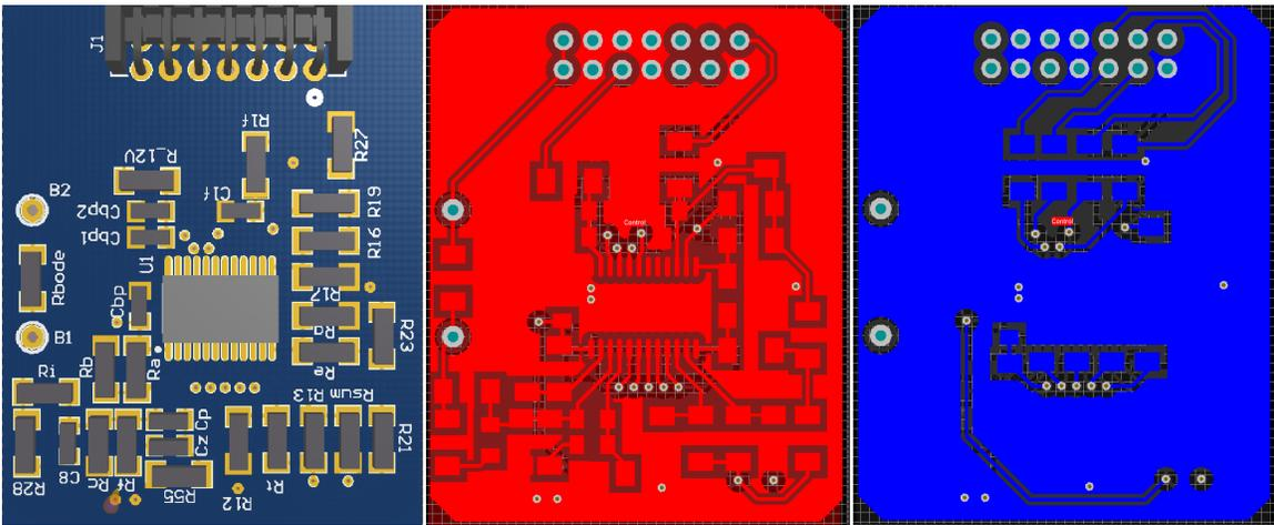
Figure 5-6: Control PCB layout on Altium Designer (3D, top, bottom)
