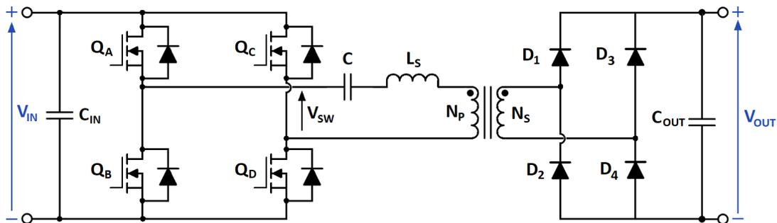
Figure 2-2: Full-bridge LLC resonant converter
