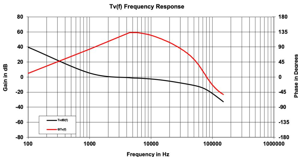
Figure 3-6: The theoretical frequency response of the converter
