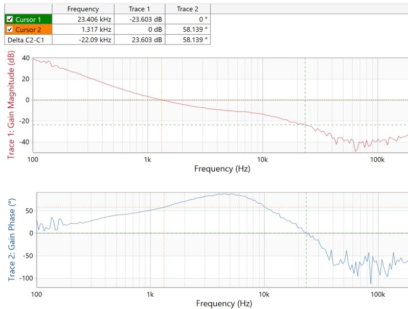
Figure 6-11: Bode analyzer loop stability test results
