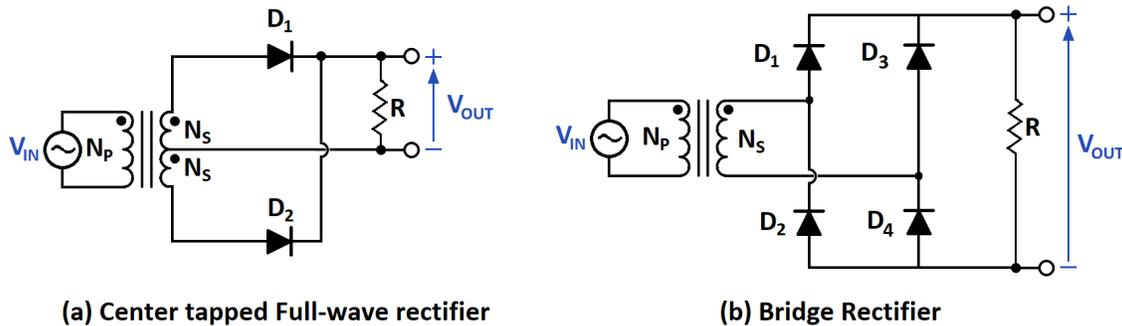
Figure 2-7: Center-tapped vs. Bridge rectifier
