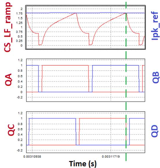
Figure 2-19: PSFB: Peak current mode control waveforms
