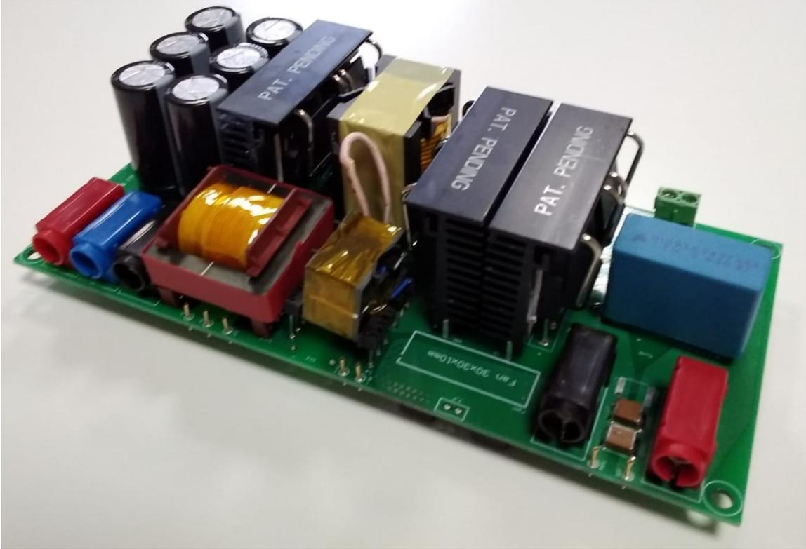
Figure 5-1: Assembled 600W power supply PCB
