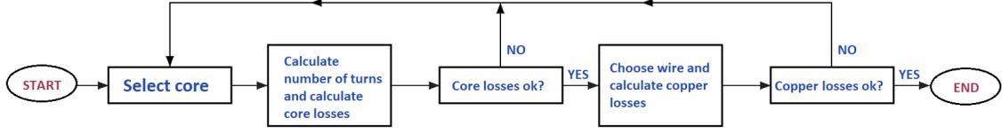
Figure 3-1: Flow chart of magnetic component design procedure
