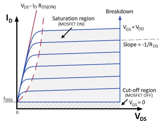
Figure 1-2: Regions of the FET transistor on the IV
