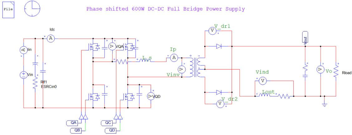
Figure 4-1: Simulation-1: Power stage
