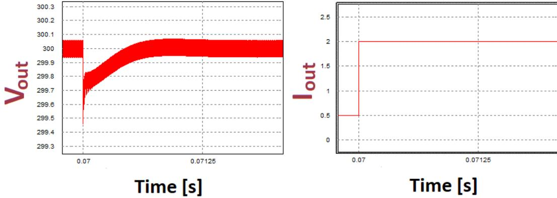
Figure 4-12: 25% to 100% load step response
