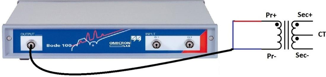
Figure 5-8: Measuring impedance using Bode 100
