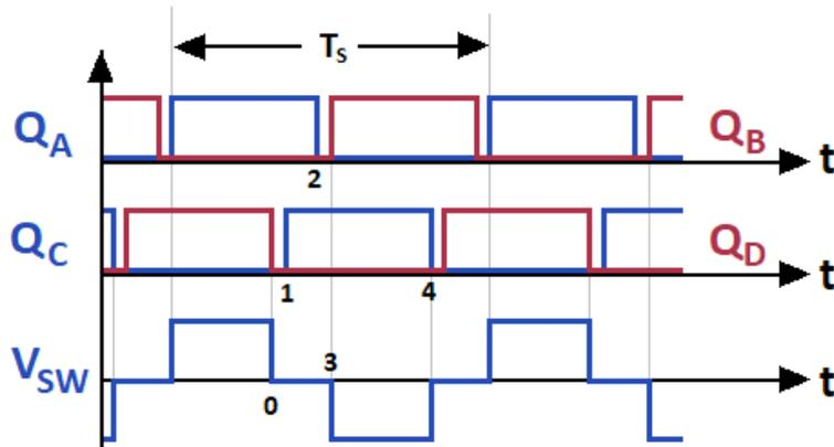
Figure 2-6: Simplified waveforms of Phase-Shifted Full-bridge converter
